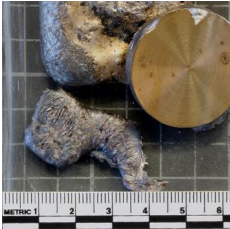
Figure 6: Metal phase of the heavy fraction after melting
