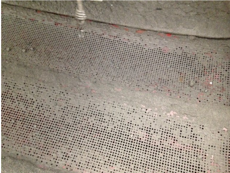
Figur 16 Delvist tilstoppet sigtesold (blinding)
