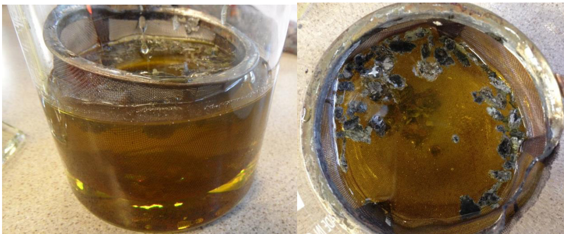
Figure 5: Light and heavy particles in sodium-polytungstate
